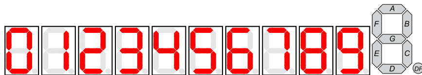
Figure 1: 7 Segment Representations of Each Integer
