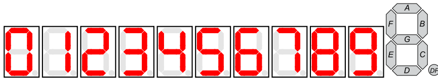
Figure 1: 7 Segment Representations of Each Integer
