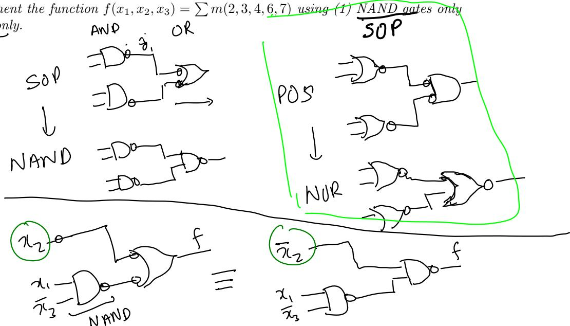
**Remark 1.** NAND-NAND logic is generated from SOP form. NOR-NOR logic is generated from POS form.
