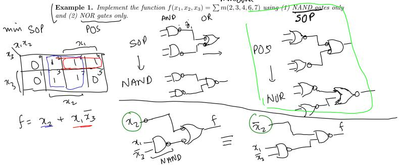
**Remark 1.** NAND-NAND logic is generated from SOP form. NOR-NOR logic is generated from POS form.
