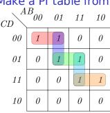
Example 5. Make a PI table from the K-map and reduce the PI table to get min-SOP form  $AB_{00}$   $B_{01}$   $B_{00}$   $B_{01}$   $B_{00}$   $B_{01}$   $B_{00}$   $B_{00}$
