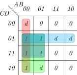
Example 6. Reduce the following PI table and find the minimal SOP form
