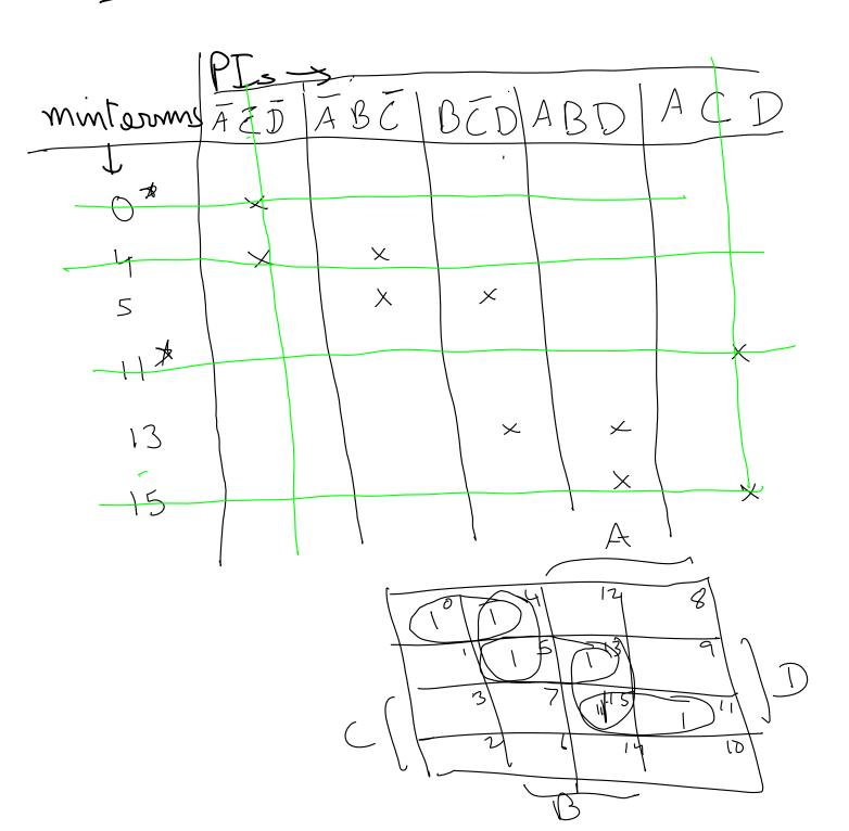
(1) Fund/gremove EPIS  $= \{ \bar{A} \bar{C} \bar{D}, ACD \}$ BED ABD ABC 2) Remove dominating trows (3) Remove dominated columns BCD donmates ABC 11 ABD (1) Find secondary FPIs = EBZDBg f=AZD+ACD+BZD J min SOP Example 5 Constant PI table and then reduce it OFINAINS PI don't cares = mmtorms (2) Finding Cover exclude 1 don't carry
