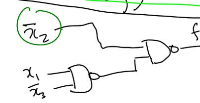
**Remark 1.** NAND-NAND logic is generated from SOP form. NOR-NOR logic is generated from POS form.
