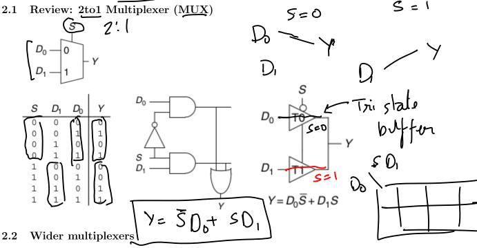
Draw the symbol for a 4:1 MUX, an 8:1 MUX and a  $2^N:1 \text{ MUX}$  and write corresponding Boolean expressions.
