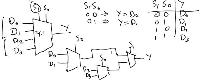
only I initems Y = 5, 50 D can be true + S, S, D, at a time. + S, & D2 The menter on that +5,50 D3 is true, selects the data line Minterms:  $\overline{S_1}$ ,  $\overline{S_0}$ ,  $\overline{S_$ The minterm that is true, selects the corresponding data line. 8:1 MUX Draw a symbol, write an expression and T How many select lines! Y= 525, So Do + 5,5, S, D, 5, 5, 50
