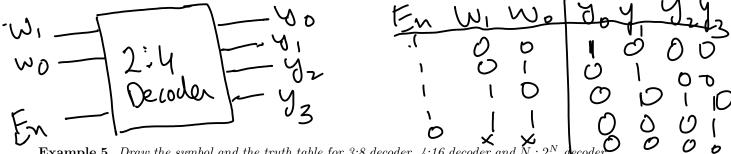
**Example 5.** Draw the symbol and the truth table for 3:8 decoder, 4:16 decoder and  $N: 2^N$  decoder. Also write the logic expressions.
