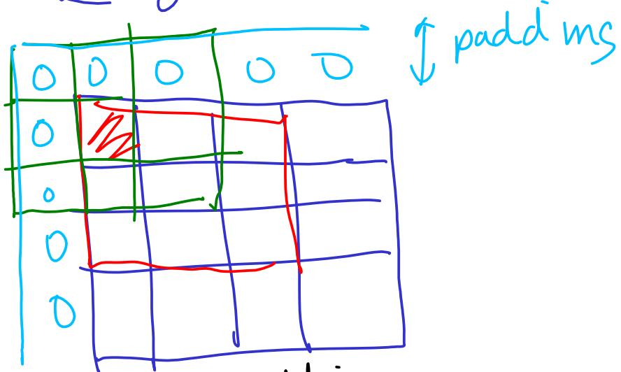
$$\begin{aligned} (4 \times 4) \text{ image} &\xrightarrow{\text{padding } \doteq 1} (6 \times 6) \text{ image} * (3 \times 3) \text{ kernel} \\ &= (4 \times 4) \text{ output} \end{aligned}$$
